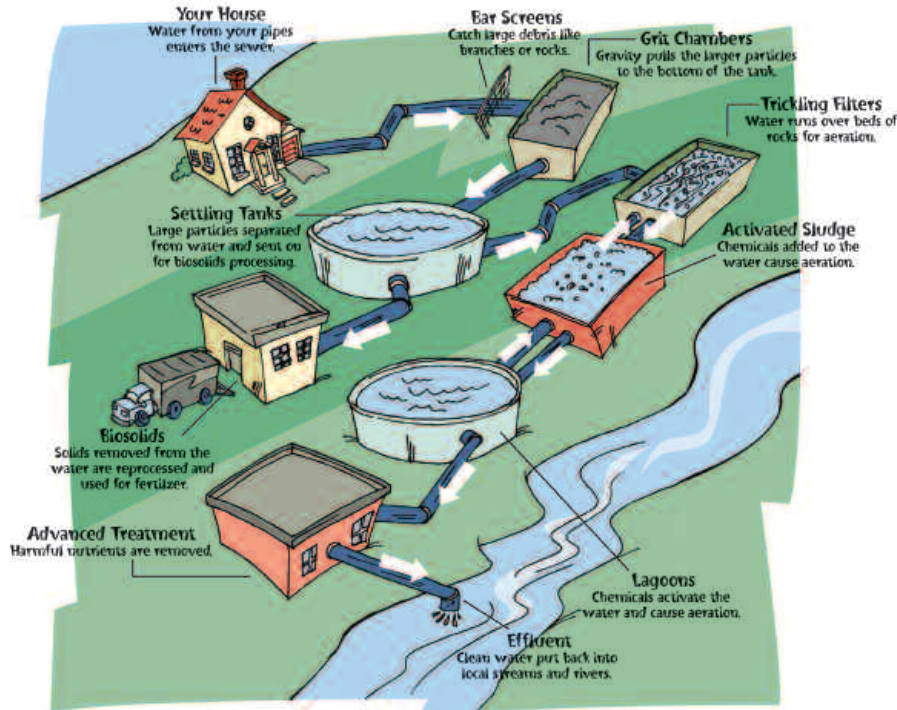
Primary Treatment Secondary Treatment Advanced Treatment Grit Chambers Trickling Filters Advanced Treatment Settling Tanks Activated Sludge Effluent Biosolids Lagoons
